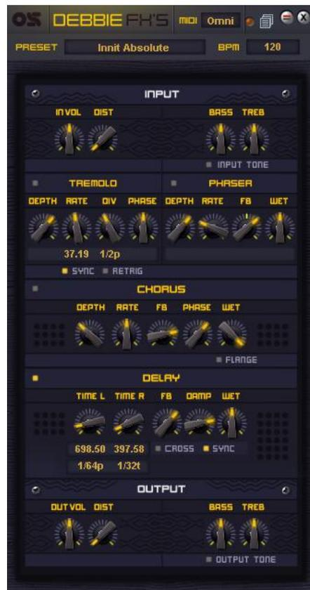
An effects box in a mono-to-stereo configuration for use with the Debbie synths or otherwise. Each effect can be bypassed. The signal chain:
