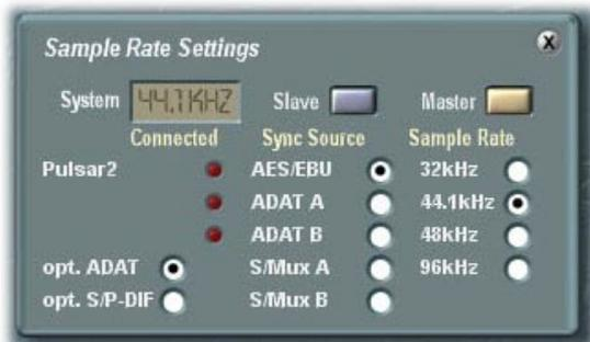
**System:** Displays the current system sampling frequency.
