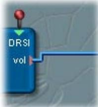
The blue wire symbolizes a synchronous connection whereas the green wire represents an asynchronous connection.
