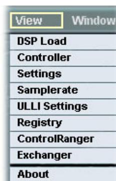
**DSP Load:** Opens or closes the DSP utilization display which monitors current DSP usage.
