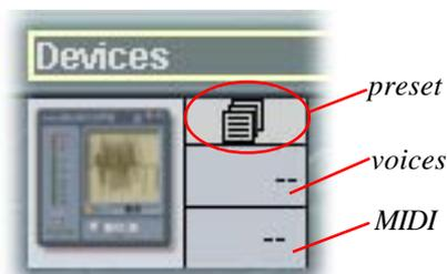
If the device is a synthesizer, the current polyphony setting is displayed below the thumbnail. This setting can likewise be altered by entering a new value.
