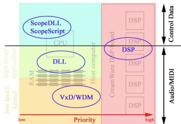
SCOPE is a DSP-based development platform. Basically you can say that the more timing is a concern the more likely the algorithm is performed on the DSPs of the CreamWare hardware.
